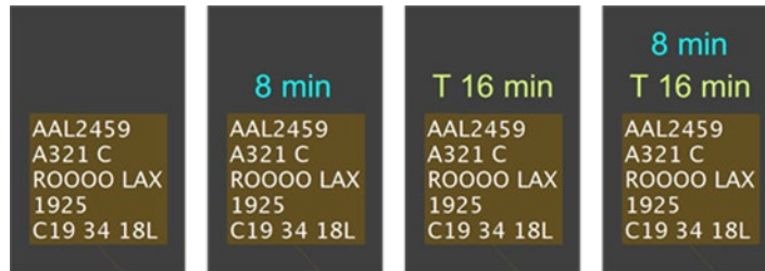
Fig. 1. TOBT and TMAT Advisories were shown in the form of countdown timers on the new ATD-2 ramp controller decision support tool, the Ramp Traffic Console (RTC). From left to right they are 1) baseline, no advisories, aircraft information only, 2) gate advisory (TOBT) shown in cyan (“8 min”), 3) spot advisory (TMAT) shown in green (“T 16 min”), and 4) both gate and spot (TOBT+TMAT) advisories displayed.
